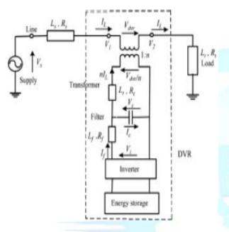
Fig.2 Distribution system with the DVR
