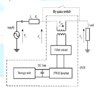
Fig.1Typical DVR-connected distribution system
