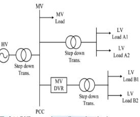
Fig.3 (a) DVR connect in a medium-voltage level power system
